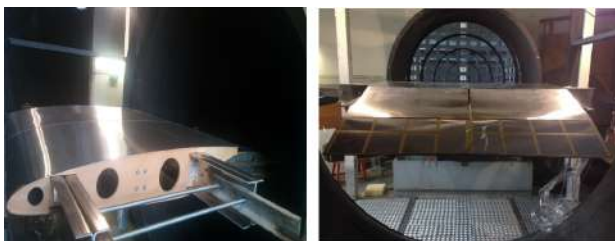
Figure 4: Morphing high-lift LS prototype of the A320 wing near scale 1 in the S1 wind tunnel of IMFT
