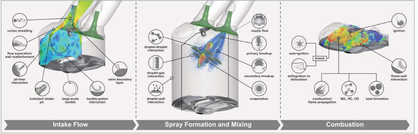
Figure 1: Cause-and-effect chain in an internal combustion engine. Individual unit problems for the computational simulation are highlighted [1]. The focus of this article is especially on the flow phenomena depicted in the left subfigure (Intake Flow)
